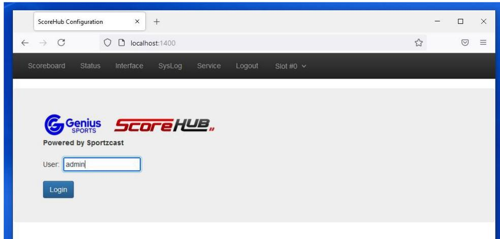
**5C.** Select the “**Interface**” tab to connect to your ScoreLink2 device. On the screen that appears, click the “**Scan for ScoreLinks**” button to locate any available Sportzcast devices on your network.
